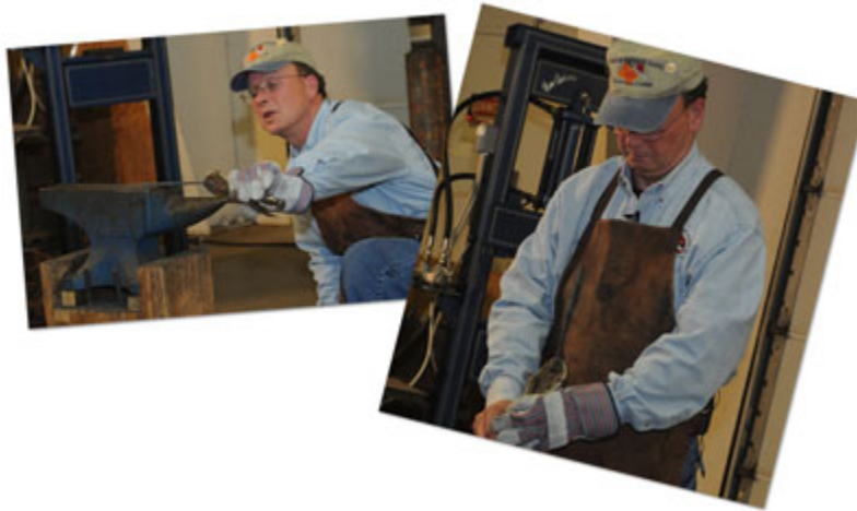
Master Smith Greg Neely checking the forged blade for straightness.
