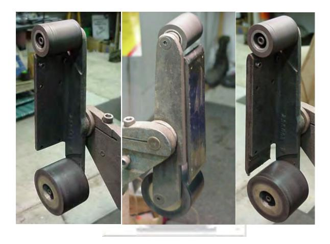
Finally.....Platens can be made in different lengths, for various applications. Like....
