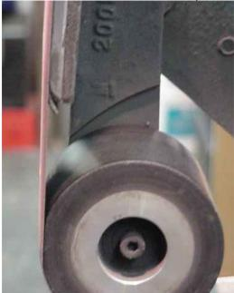
I seldom use the 8" wheel, with the exception of profiling blades. The long flat platen, I use for flattening, and tapering, the shorter platen is used for convex grinding.
